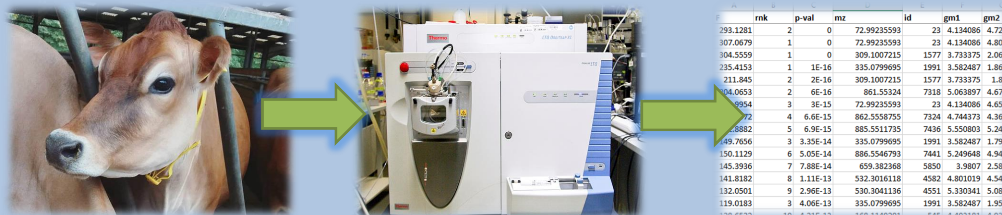
Figure 3 – The process of producing metabolomic data. Following collection, samples are processed using the flow-infusion electrospray-mass spectrometry on the exactive orbitrap MS platform before being statistically analysed.
